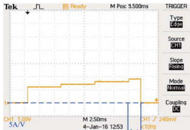
Figure 5-22 3356G BMS Overcharge flow Test Results (Continuous STEP Pulse)
