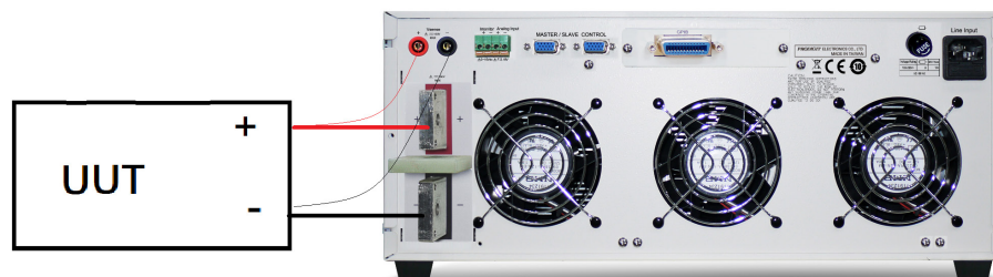
Fig 5-2 Remote voltage sense connections
