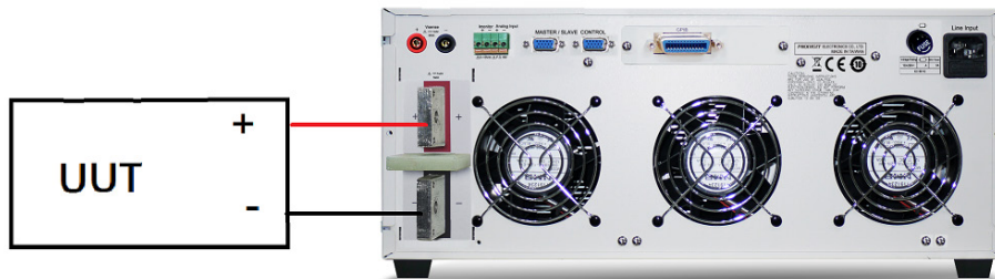
Fig 5-1 Local voltage sense connections
