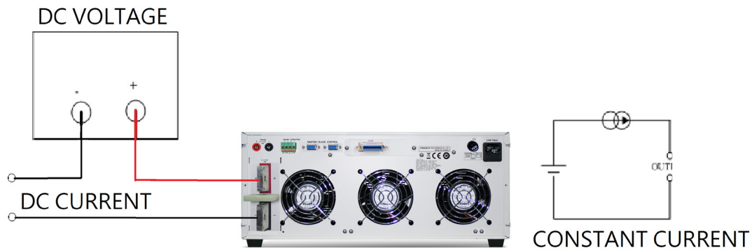
Fig 5-10 constant current source connection
